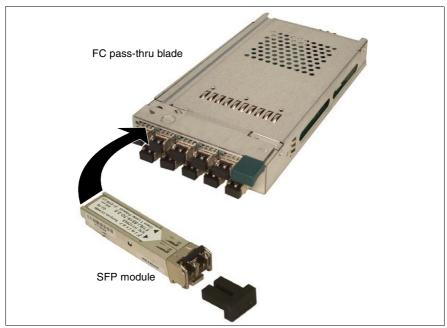
Figure 52: Fibre Channel pass-thru blade
